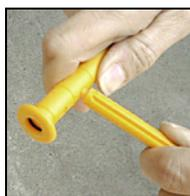
If isolated measurements in the 1/2 in. (13 mm) to 2 1/2 in. (64 mm) depth range are required, use the sleeve tool to knock out both windows in the appropriate section only. If isolated measurements are required at depths exceeding 2 1/2 in. (64 mm), use the sleeve tool to knock out the window in the base of the sleeve (see photo at right).
