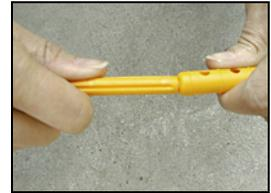
If a measurement is required across the entire length of the humidity sleeve, use the sleeve tool to knock out all of the windows in all four sections of the sleeve.
