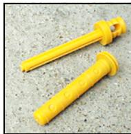
The *humidity sleeve tool* (top item in photo above) is used to knock out the windows and to drive the sleeve fully into the pre-drilled clearance holes. The tool should always be used for this purpose to ensure that the sleeve is not damaged during placement.
