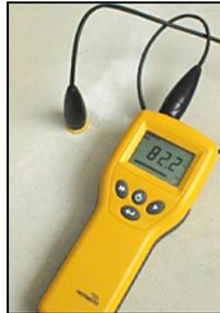
**Note:** *It is possible to connect the Hygrostick directly to the instrument, but it is preferable to use the Hygrostick extension lead (part number BLD5802).*
